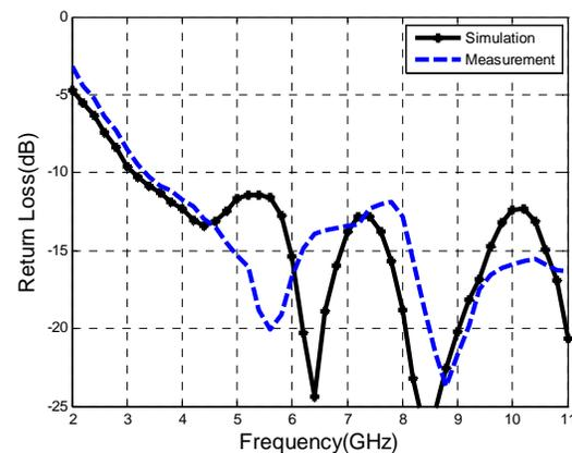
Fig.5 Variation of the measured and simulated return loss with frequency.
