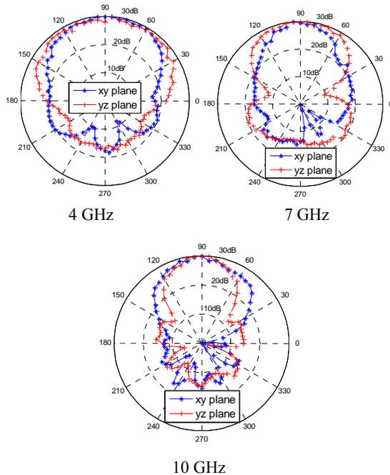
Fig.6 The measured radiation pattern three frequencies.
