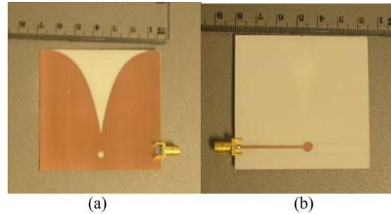
Fig.4 The manufactured antenna. (a) Top layer revealing the radiator and the transition, and (b) bottom layer showing the microstrip feeder.
