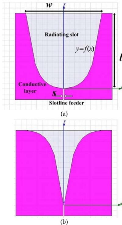
Fig.1 The tapered slot antenna. (a) Positive tapering, and (b) negative tapering.
