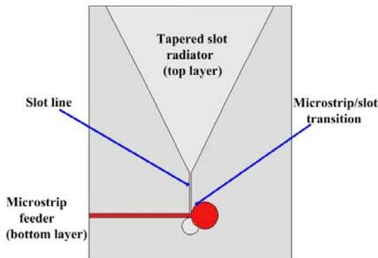
Fig.3 Configuration of the microstrip/slot line transition as a method to feed the antenna using a microstrip line.
