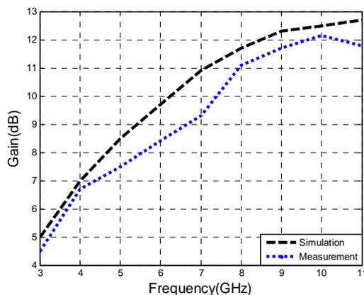
Fig.7 Variation of the measured and simulated gain with frequency.
