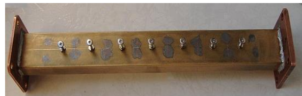
Fig.6. Fabricated waveguide bandpass filter with dual post obstacle
