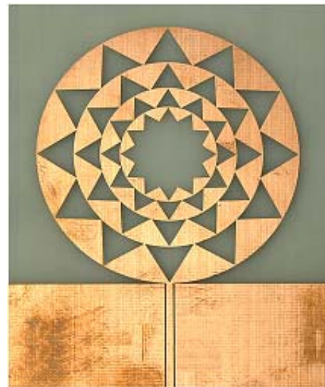
Fig. 4. Photograph of the Triangular Wheel Shape Fractal Antenna
