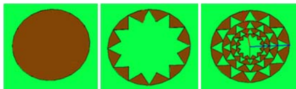
(a) Fig. 1. Circular Microstrip Patch (b) Fig. 1. 1 st iterative Antenna (c) Fig. 1 4 th iterative Fractal Antenna
