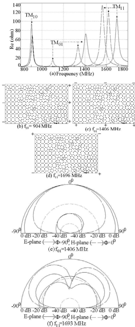
Fig. 4 (a) Resonance curve plots for (—) RMSA, (---)  $l = 1.0$  cm, (----)  $l = 2.0$  cm, (b – d) surface current distribution and (e, f) radiation pattern at various modes for RMSA
