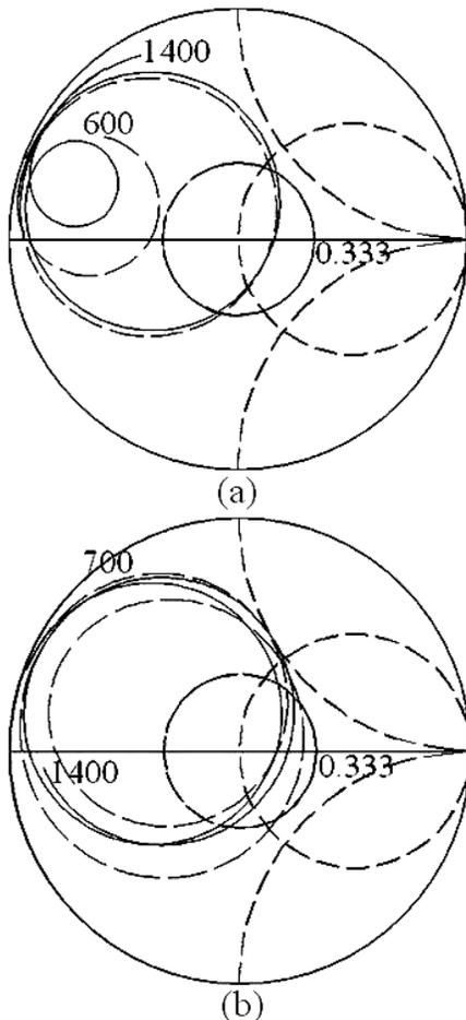
Fig. 2 Measured input impedance plots for dual band RMSA shown in (a) Fig. 1(a), (—)  $l = 2$  cm, (---)  $l = 5$  cm, and (b) Fig. 1(b), (—)  $l = 2$  cm, (---)  $l = 5$  cm
