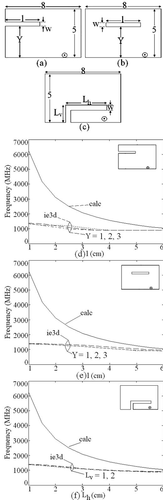
Fig. 1 Dual band (a, b) rectangular slot and (c) half U-slot cut RMSAs and its (d – f) frequency and % error plots
