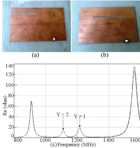
Fig. 3 (a, b) Fabricated prototype of dual band RMSAs and (c) resonance curve plot for different Y for dual band RMSA shown in Fig. 1(a)
