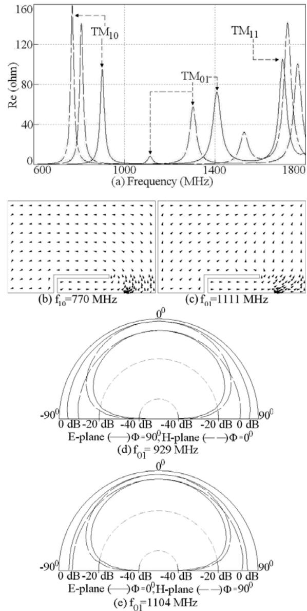
Fig. 7 (a) resonance curve plot for half U-slot cut RMSA, (—) RMSA, (— —)  $L_h = 2.0$ ,  $L_v = 1.0$ , (---)  $L_h = 3.0$ ,  $L_v = 1.0$ , and its (b, c) surface current distribution at dual frequencies,  $L_h = 3.0$ ,  $L_v = 1.0$ , radiation pattern for (d) rectangular slot ( $l = 5$  cm) and (e) half U-slot cut ( $L_h = 3.0$ ) RMSA at  $TM_{01}$  mode
