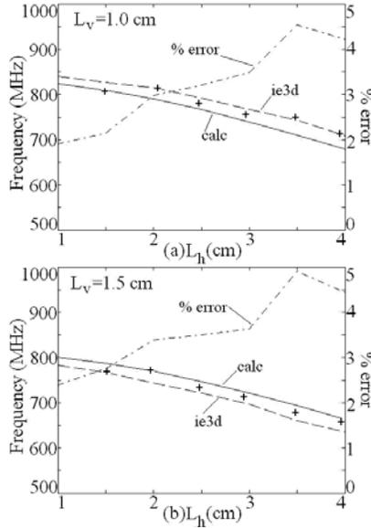
Fig. 12 (a, b) Resonance frequency and % error plots at TM<sub>10</sub> mode for half U-slot cut RMSA, (+ + +) measured
