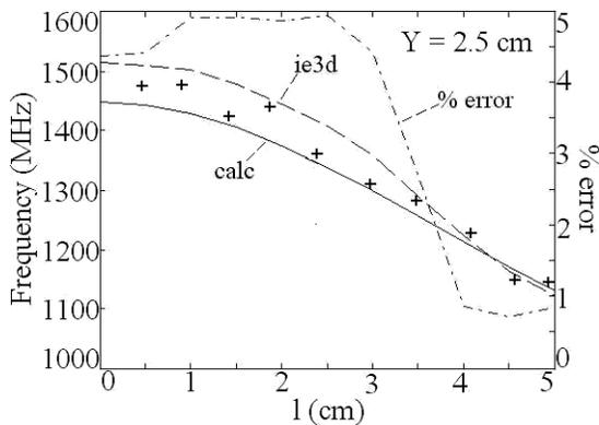
Fig. 16 Resonance frequency and % error plots for half U-slot cut RMSA with rectangular slot cut inside the patch at  $TM_{11}$  mode, (+ + +) measured
