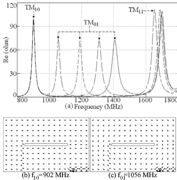
Fig. 6 (a) Resonance curve plots for rectangular slot cut RMSA shown in Fig. 1(b), (—)  $l = 0$ , (— —)  $l = 2$ , (---)  $l = 3$ , (— · —)  $l = 4$ , its (b, c) surface current distribution at dual frequencies,  $l = 4$
