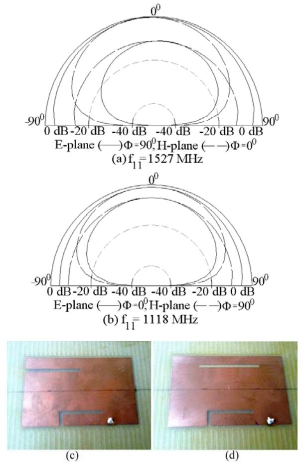
Fig. 9 Radiation pattern at modified  $TM_{11}$  mode for triple band RMSA shown in Fig. 8(b) for (a)  $l_1 = 0$  and (b)  $l_1 = 4$  cm, (c, d) fabricated prototypes of triple band RMSA
