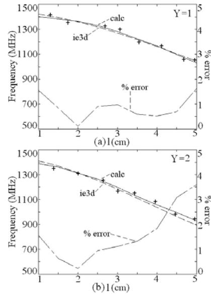
Fig. 11 (a, b) Resonance frequency and % error plots for rectangular slot cut inside RMSA, (+ + +) measured
