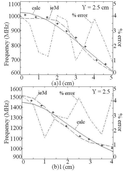
Fig. 14 Resonance frequency and % error plots at (a)  $TM_{01}$  and (b)  $TM_{11}$  modes for half U-slot and rectangular slot cut RMSA, (+ + +) measured
