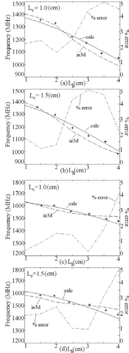
Fig. 13 Resonance frequency and % error plots at (a, b) TM<sub>01</sub> and (c, d) TM<sub>11</sub> mode for dual band half U-slot cut RMSA, (+ + +) measured
