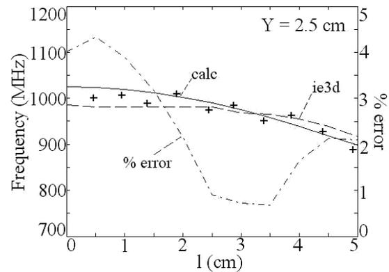
Fig. 15 Resonance frequency and % error plots for half U-slot cut RMSA with rectangular slot cut inside the patch at  $TM_{01}$  mode, (+ + +) measured
