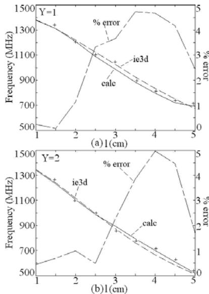
Fig. 10 (a, b) Resonance frequency and % error plots for rectangular slot cut RMSA, (+ + +) measured
