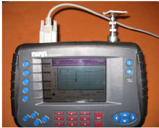
Fig.7. Photograph of experimental set up to test metamaterial loaded polypropylene based wearable T-shaped microstrip patch antenna
