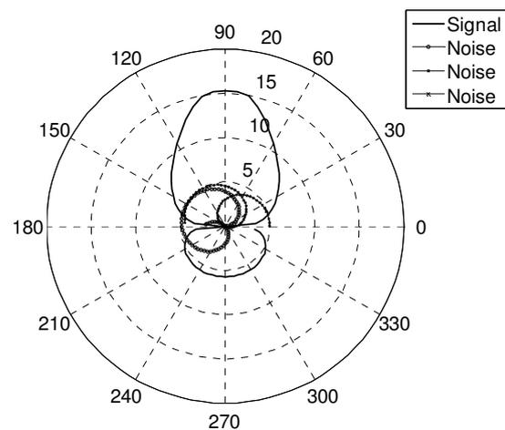
Fig. 4 Radiation pattern of array antenna with noise suppression
