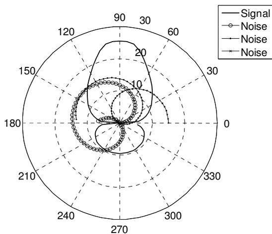
Fig. 3 Radiation pattern of array antenna with noise
