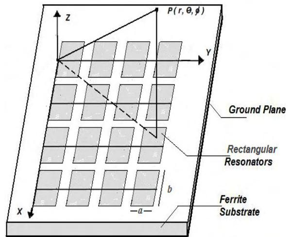
Fig: 1 Schematic diagram of antenna array of 16 elements
