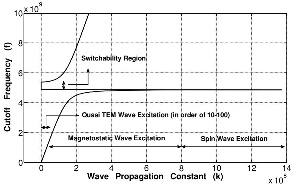
Fig. 2: Dispersion curve (f vs. k) of MSW in LiTi for incident plane wave perpendicular to the biased substrate by 750 Oe. magnetic field.
