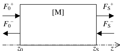
Fig. 1. Schematic representation of the relationship between input and output fields at both ends of an active structure.
