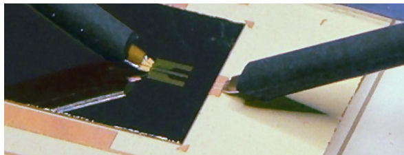
Fig. 11. Photograph of single coupler prototype with on-wafer probes
