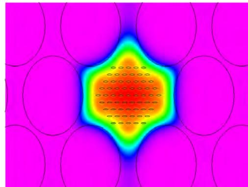
Fig.2. The profile of the major electric field component of the y-polarized fundamental mode at a normalized frequency 1.
