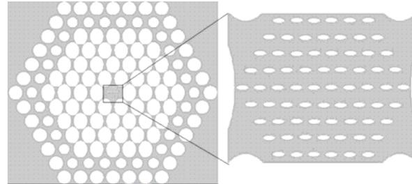
Fig. 1. Schematic diagram of the proposed PCF with four rings of elliptical air holes and the two outermost rings of circular air holes in the fiber cladding and the elliptical air  $\mu$ -holes in the fiber core.
