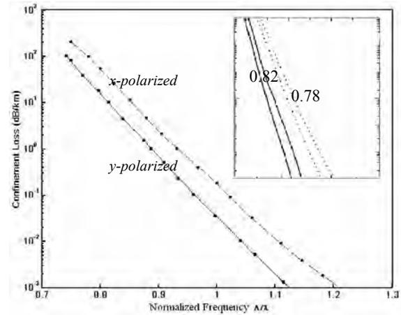
Fig.4. Confinement losses of the  $x$ -polarized (filled circles with dashed line) and the  $y$ -polarized (filled square with solid line) of the fundamentals modes for the proposed PCF as a function of normalized frequency. Inset shows the confinement losses for  $e=0.78$  (dotted line) and  $e=0.82$  (solid line)
