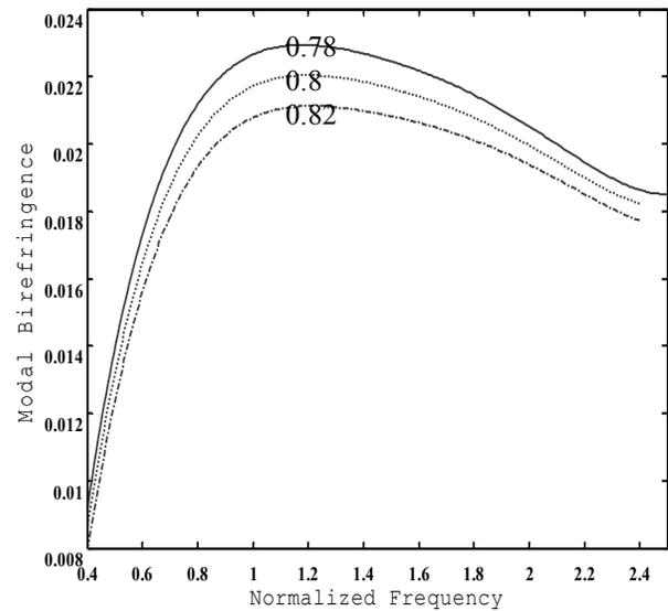
Fig.5. Illustrate the modal birefringence of the PCF as a function of normalized frequency with varying ellipticity 'e' from 0.78 to 0.82 by an interval of 0.02.
