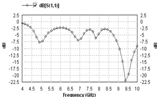
Fig.6. Return loss ( $S_{11}$ ) characteristics of unloaded rectangular slotted microstrip patch antenna on the finite ground plane
