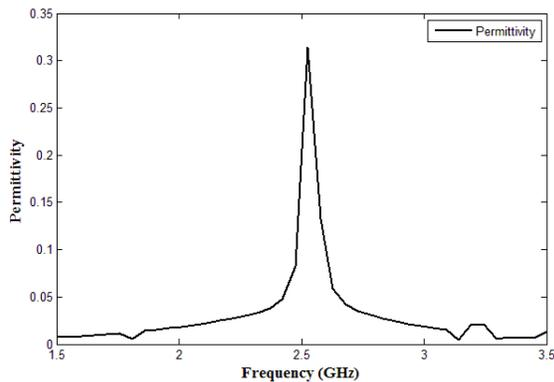
Fig.5(b). Relative permittivity ( $\epsilon_r$ ) characteristics of MSRR as a function of frequency
