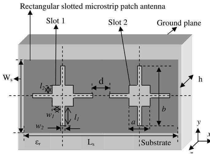
Fig. 1. Sketch and geometrical structure of rectangular slotted microstrip patch antenna
