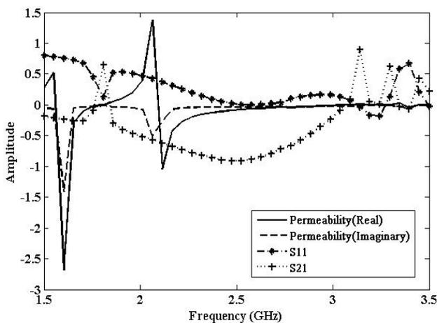
Fig.5(c). S-parameters and relative permeability ( $\mu_r$ ) characteristics of MSRR as a function of frequency
