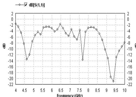
Fig.7. Return loss ( $S_{11}$ ) characteristics of metamaterial MSRR loaded rectangular slotted microstrip patch antenna on the finite ground plane
