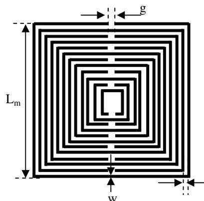
Fig.3. Geometrical structure of MSRR (Number of split rings  $N = 12$ ) etched on the ground plane
