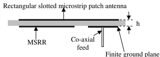
Fig.2. Cross sectional view of rectangular slotted microstrip patch antenna loaded with MSRR on the finite ground plane
