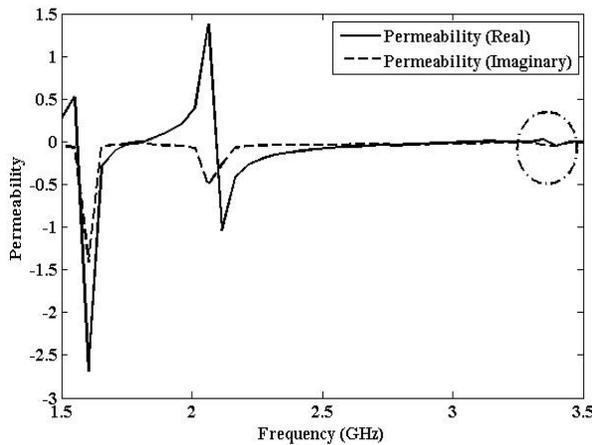
Fig.5(a). Relative permeability ( $\mu_r$ ) characteristics of MSRR as a function of frequency
