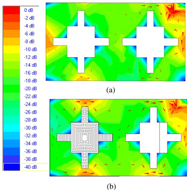
Fig.8. Simulated surface current distribution on the rectangular slotted microstrip patch (a) without MSRR loading (b) with MSRR loading conditions
