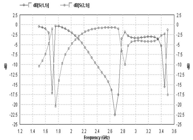
Fig. 4. Reflection coefficient ( $S_{11}$ ) and transmission coefficient ( $S_{21}$ ) characteristics of MSRR
