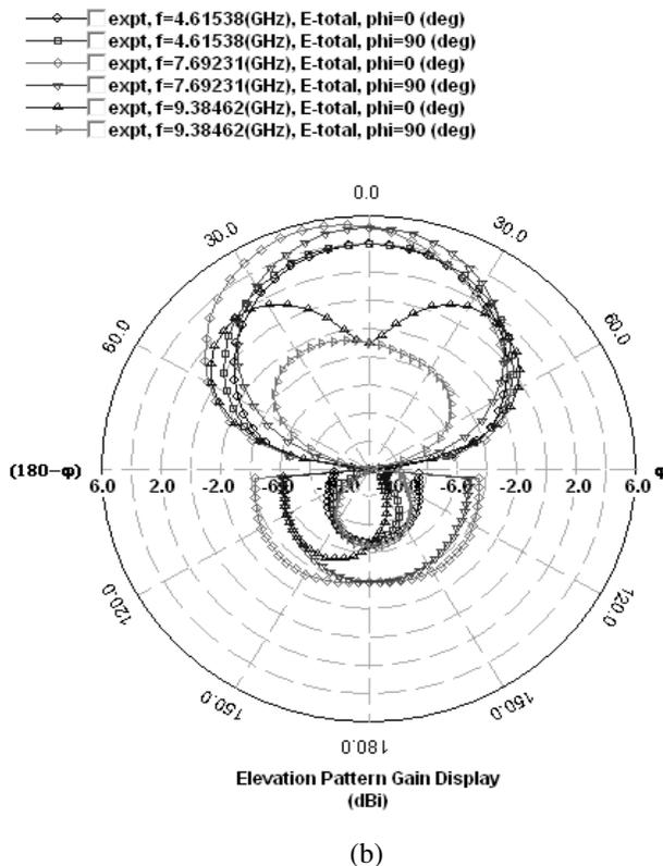
Fig.10. Radiation patterns of metamaterial MSRR loaded rectangular slotted microstrip patch antenna with finite ground plane (a) azimuth (b) elevation
