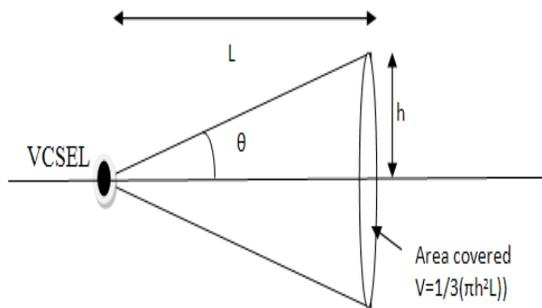
Fig 1: Single Transceiver coverage Area
