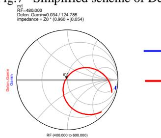
Fig.8 Delon doubler input impedance.
