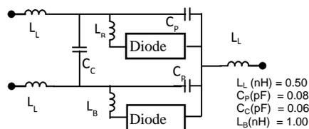
Fig.2. Model of the SOT323 package.
