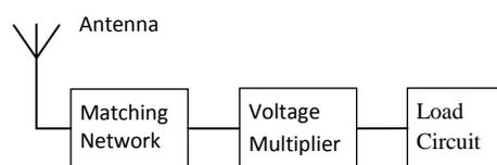
Fig.1. Block diagram of an energy harvesting system.
