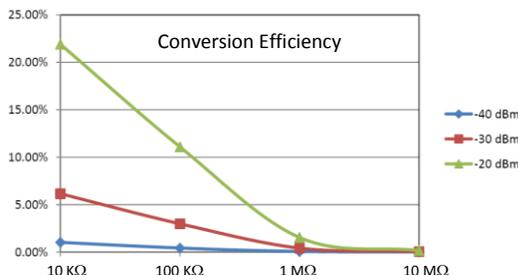
Fig.15. RF/DC conversion efficiency by Greinacher doubler.
