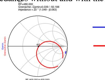
Fig.6 Greinacher doubler input impedance.
