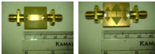
Fig. 6: Fabricated LPF (a) Top side, (b) Bottom side
