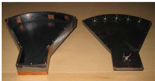
Fig.8. A picture of the opened power divider.
